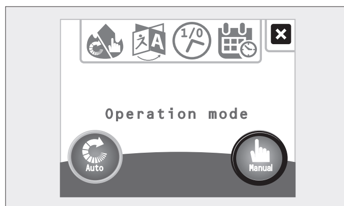
Fig. 3.20 Touch control panel – Manual operating mode
